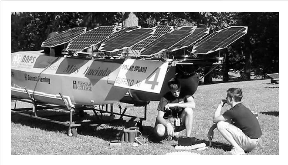
Bryan Pilcher and Andrew Bryden monitor the automatically tracking solar array as it charges the battery pack.
