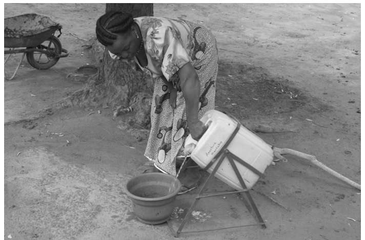
A woman with use of only one arm tests a jerry can tipper designed by the water transport team.
