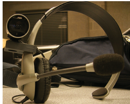
Lifecam mounted on modified headset of enhanced WERC prototype
