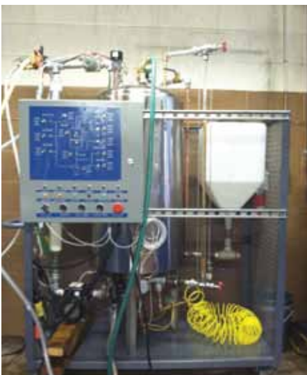
Automated biodiesel processor with engraved schematic
