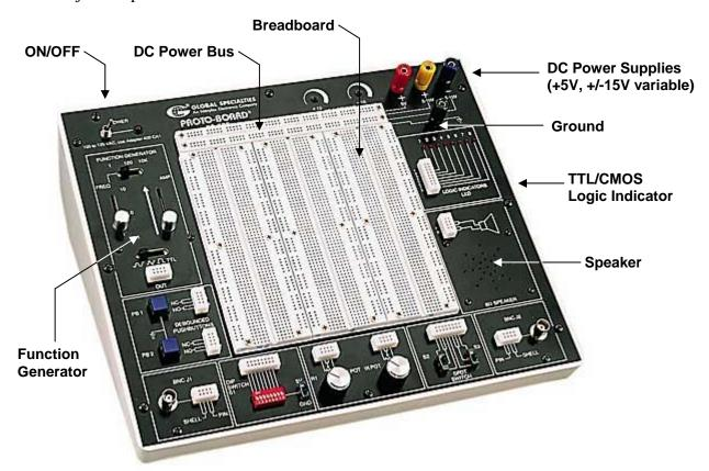
Onboard DC power is available in the top-right corner of the board and also from the power bus that runs along the top of the breadboard. In order to avoid electrocuting yourself, damaging your circuit components, or damaging the equipment, observe the following rules concerning electrical power:
