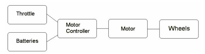
The lithium polymer battery packs were configured into a parallel and series stacks configuration. The arrangement provides the optimal voltage and current needs for our electric drivetrain system. The battery array is then connected to the motor controller. This motor controller is connected to a throttle which determines the amount of power which is sent to the motor. The final component of the electric drivetrain is the DC motor which drives the rear wheel of our motorcycle.
