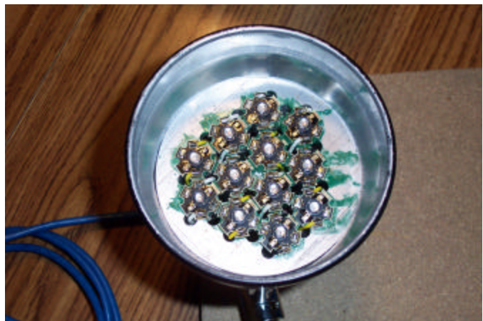
Figure 3-8: Each lighting fixture contained twelve total LEDs: four red, four green, and four blue.
