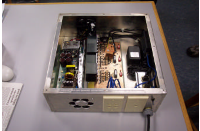
Figure 3-7: All the power and data components are fixed into a protective casing.
