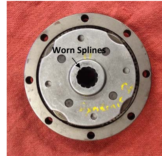
Figure 2: Worn sintered metal planetary
