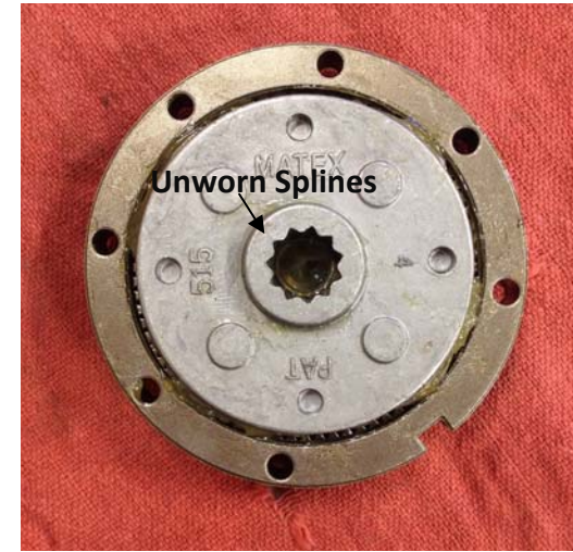
Figure 1: Unused sintered metal planetary
