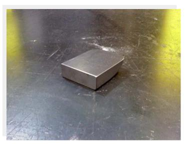
**Axle bushing** was turned on lathe to proper diameter
