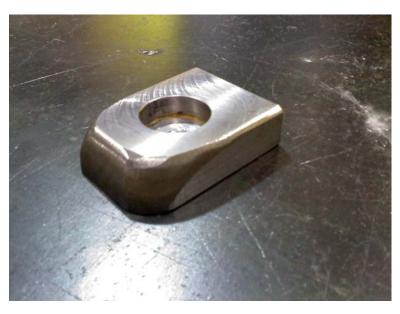
**Axle block** edge fillets were applied by hand to fit piece to swingarm location
