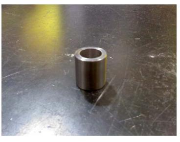
**Axle block** bushing pocket was precision milled on CNC machine
