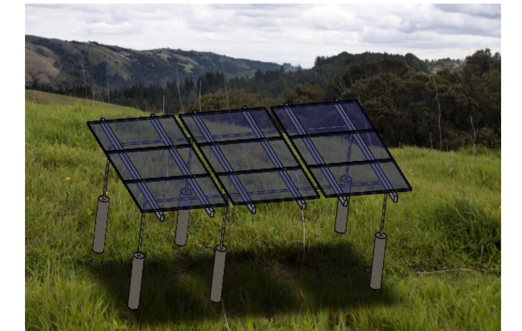
Figure 8: the nine solar panel ground mounting structure
