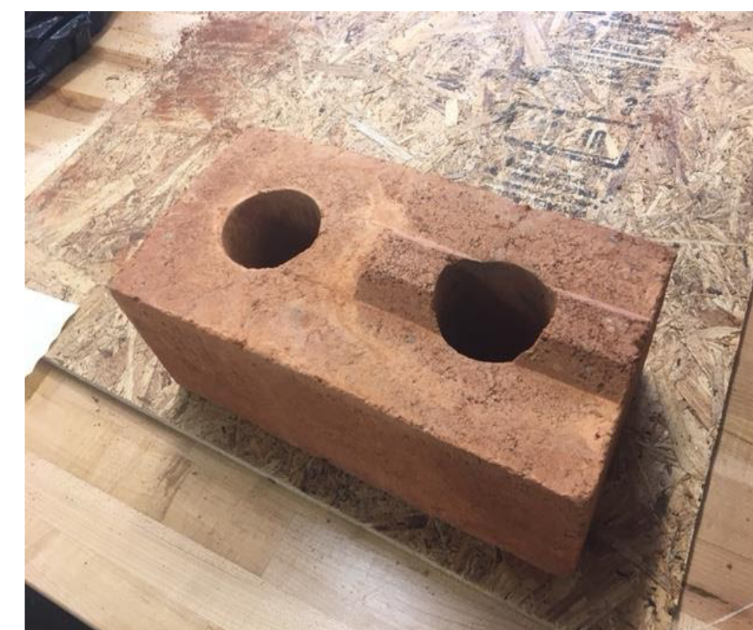
Block pressed and cured
