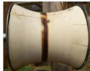
A simple wooden capstan was also tested, but it produced enough heat to quickly melt the nylon rope. The team will continue to test alternate solutions until the wear has been significantly reduced.
