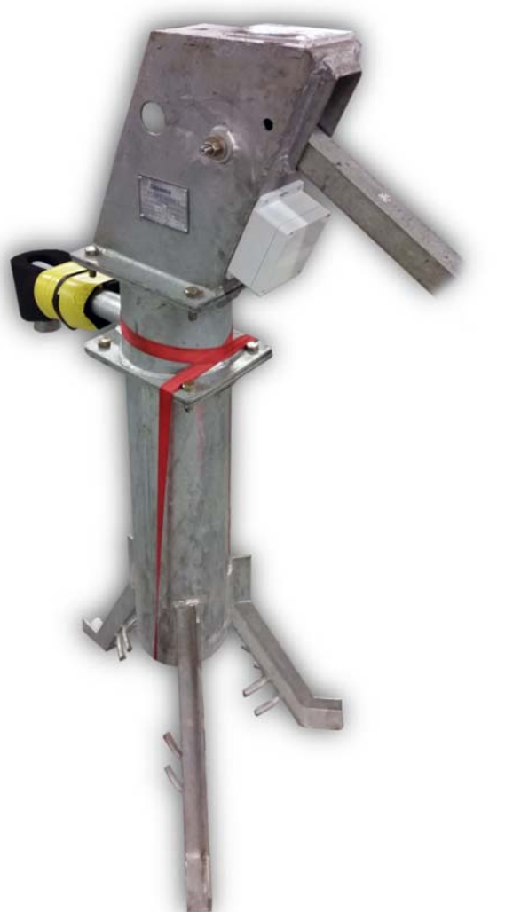
IWP system attached to hand pump
