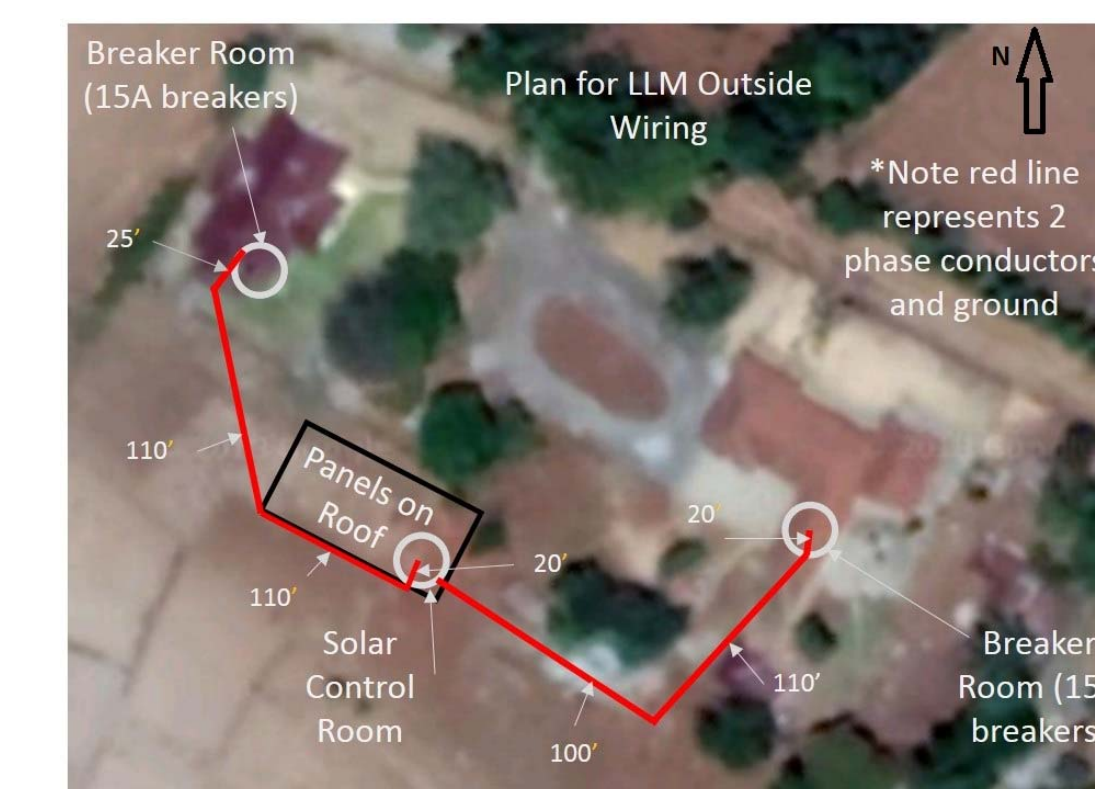
Figure 7: In-Between Building Wiring Plan
