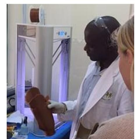
Figure 4 - One of the technicians (Shadrack) holding a printed prosthetic socket next to the 3D printer.
