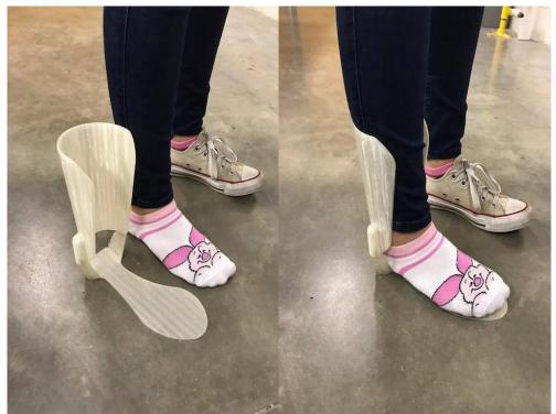
Figure 7 – Version 1 of our 3D printed Ankle-Foot Orthotic tested on a team member.
