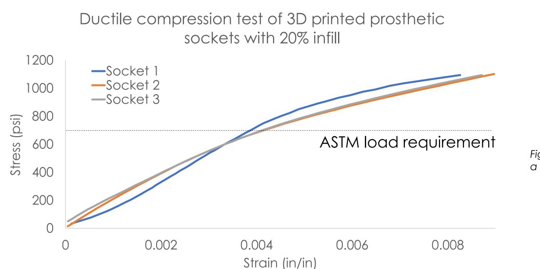
Figure 5 - - Results from the compression testing
