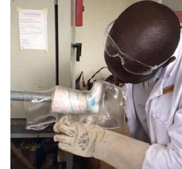
Figure 5: Current Vacuum Molding Process
