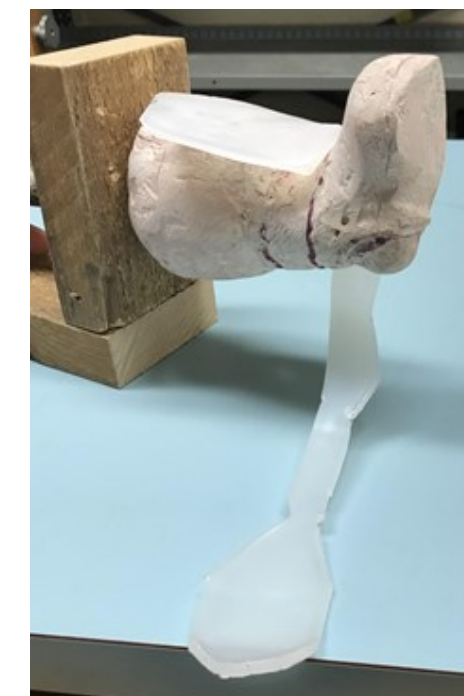
Figure 6: Wrapping Polypropylene around a mold
