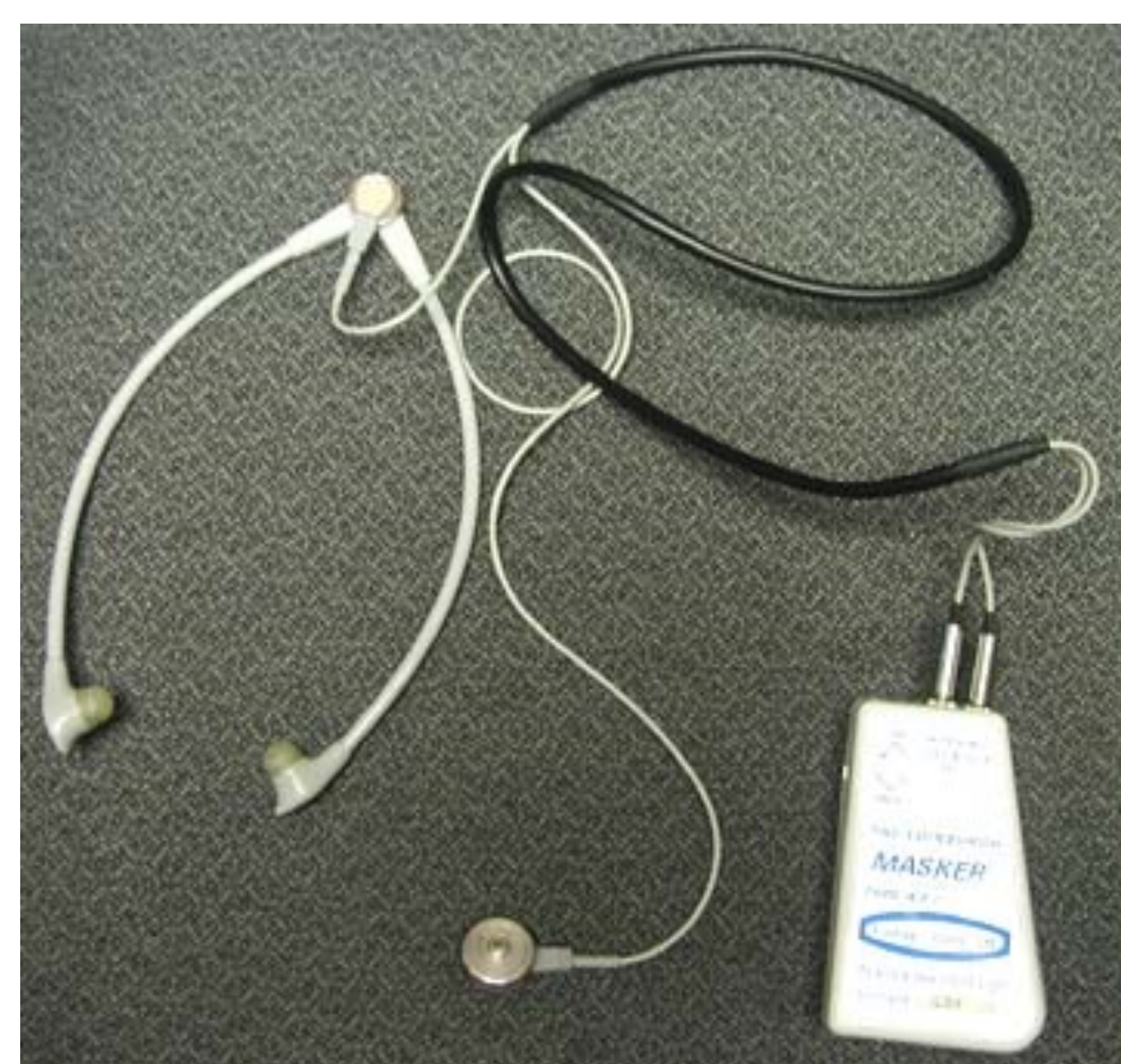
Figure 1: Original Edinburg Masker including throat microphone, headset, and electronics module.
