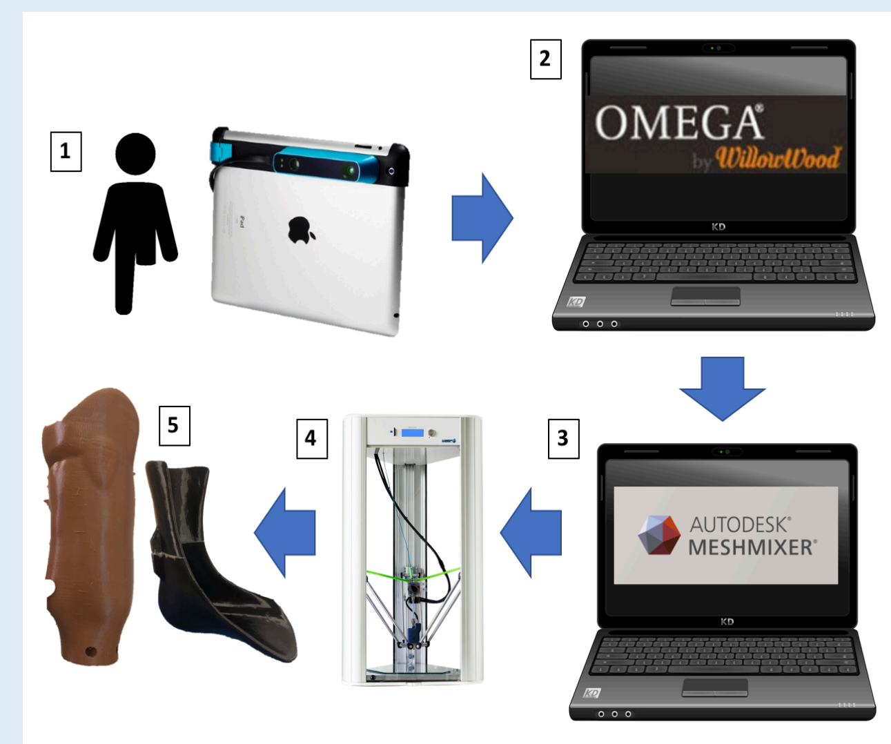
Figure 3– Current process of 3D printing system
