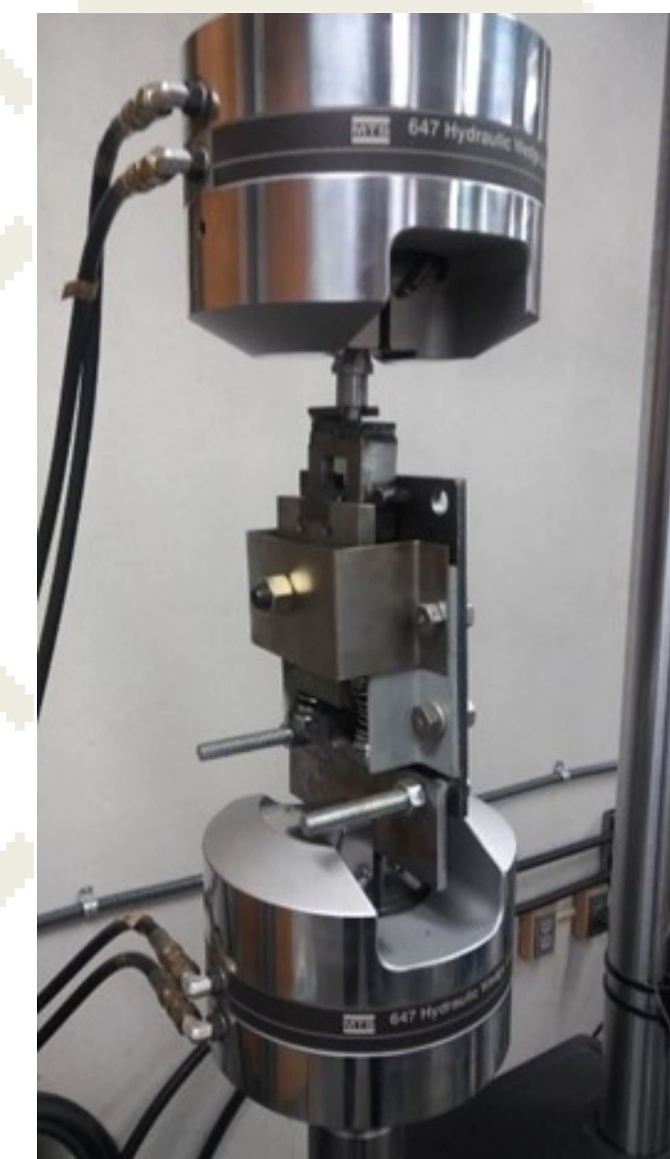
Latch prototype in the tensile tester
