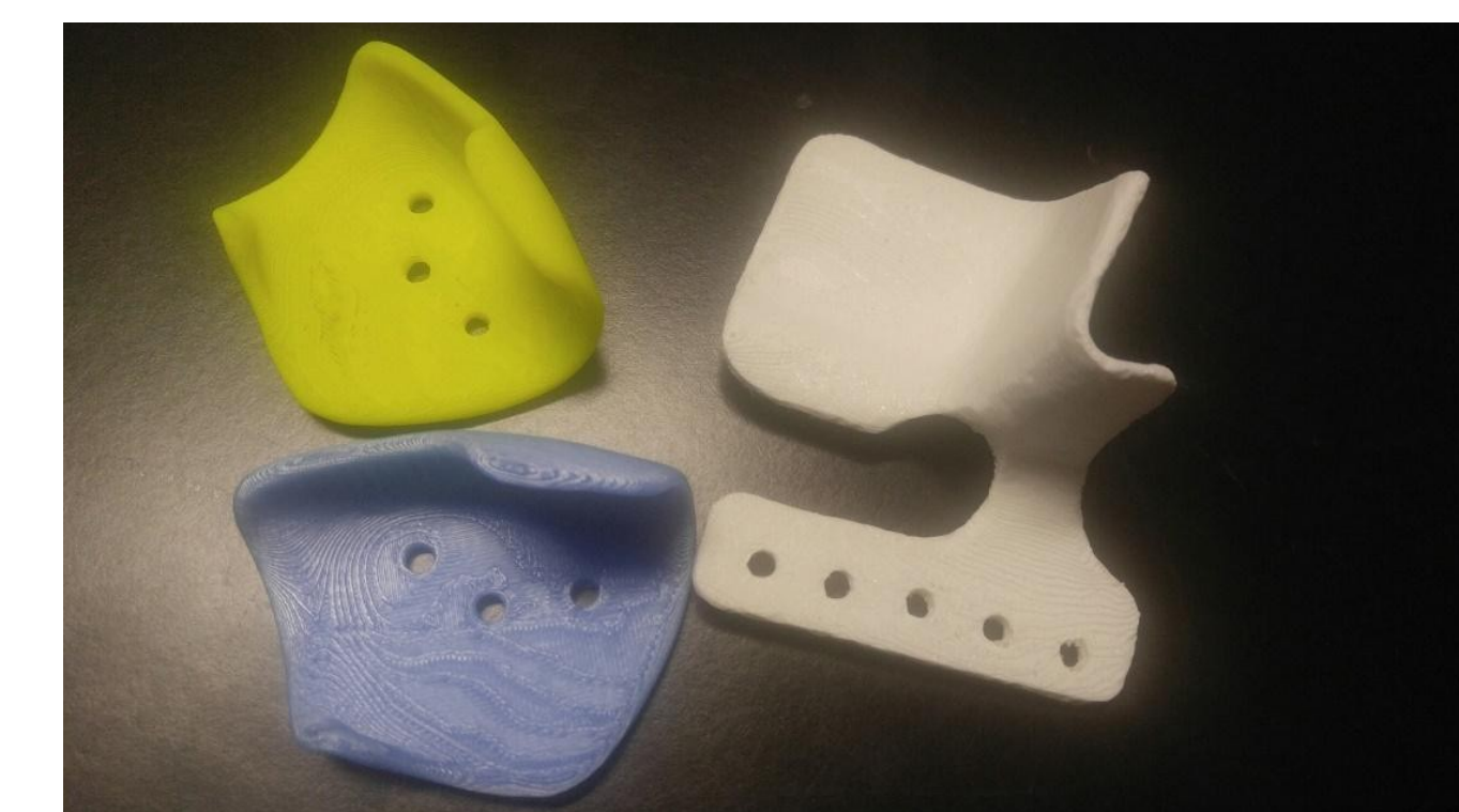
Figure 9: Prototype prints for clubfoot brace
