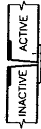
FLAT PLATE ASTRAGAL 4491 PLAIN STEEL (welded on) (Medallion & Thrulite Doors only) 4481 STAINLESS STEEL (screwed on) (Stainless steel doors only)
