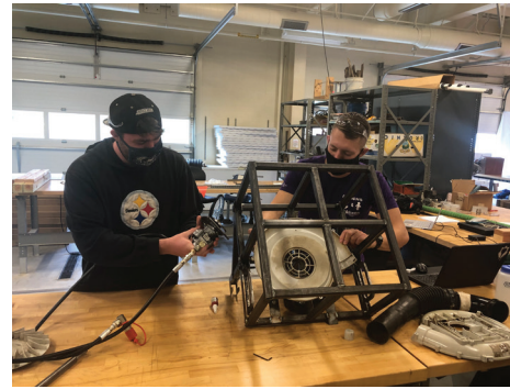
Working on placement to mount the blower and motor assembly within the protective cage
