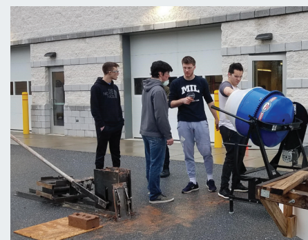
Team prepares mud to use in block press
