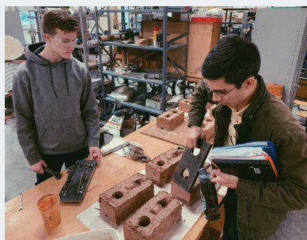
Project Manager Dr. Phillip Tan inspects block made with the press
