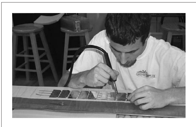
Team member Stephen Osborne '06 uses the hot nitrogen soldering iron to make final connections on a string of several solar cells.
