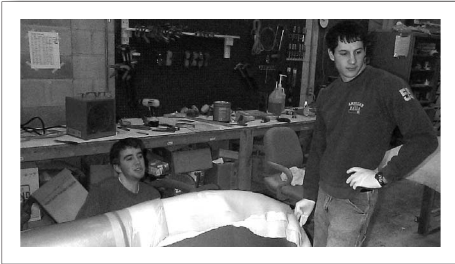
Team members Kurt Stabler '05 and Fred Yutzky '05 work on reducing drag by re-shaping the leading edges of the existing carbon fiber hull.
