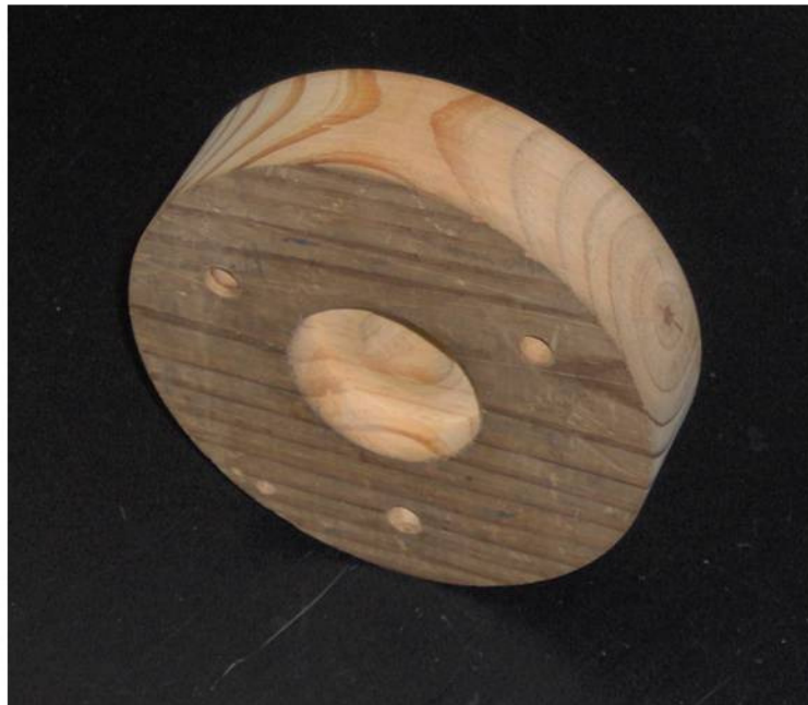
Figure 6 - Wooden propeller sprocket mock-up
