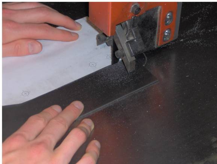
Figure 7 - Cutting the sheet metal base bracket pieces
