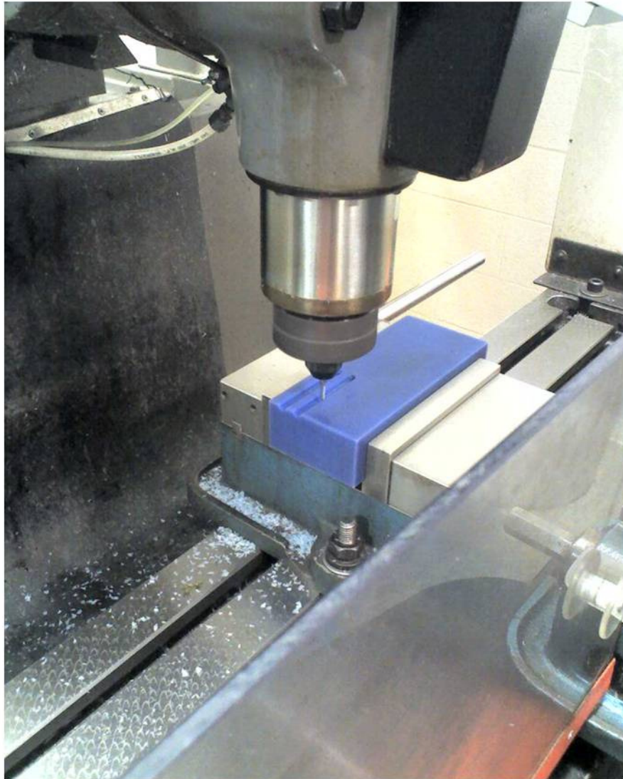
Figure 10 - Testing the propeller sprocket tooth profile CNC program
