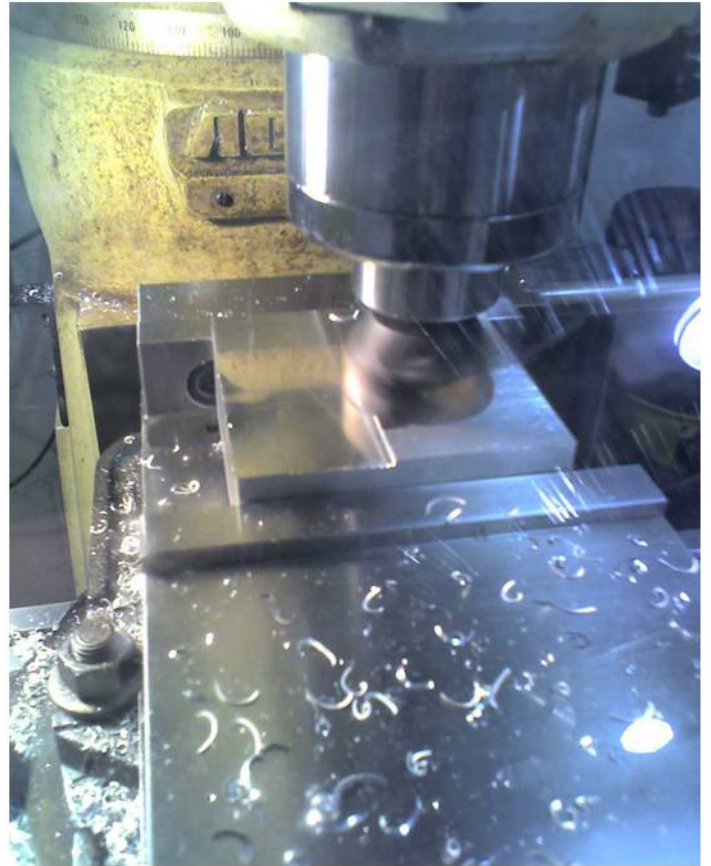
Figure 2 - Face milling a support blocks
