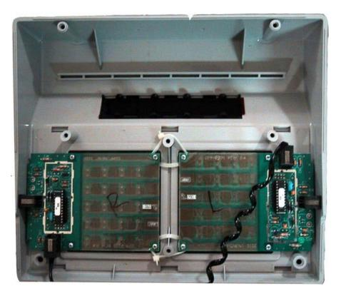
Figure 6 – Internal View of Control Box Keypad
