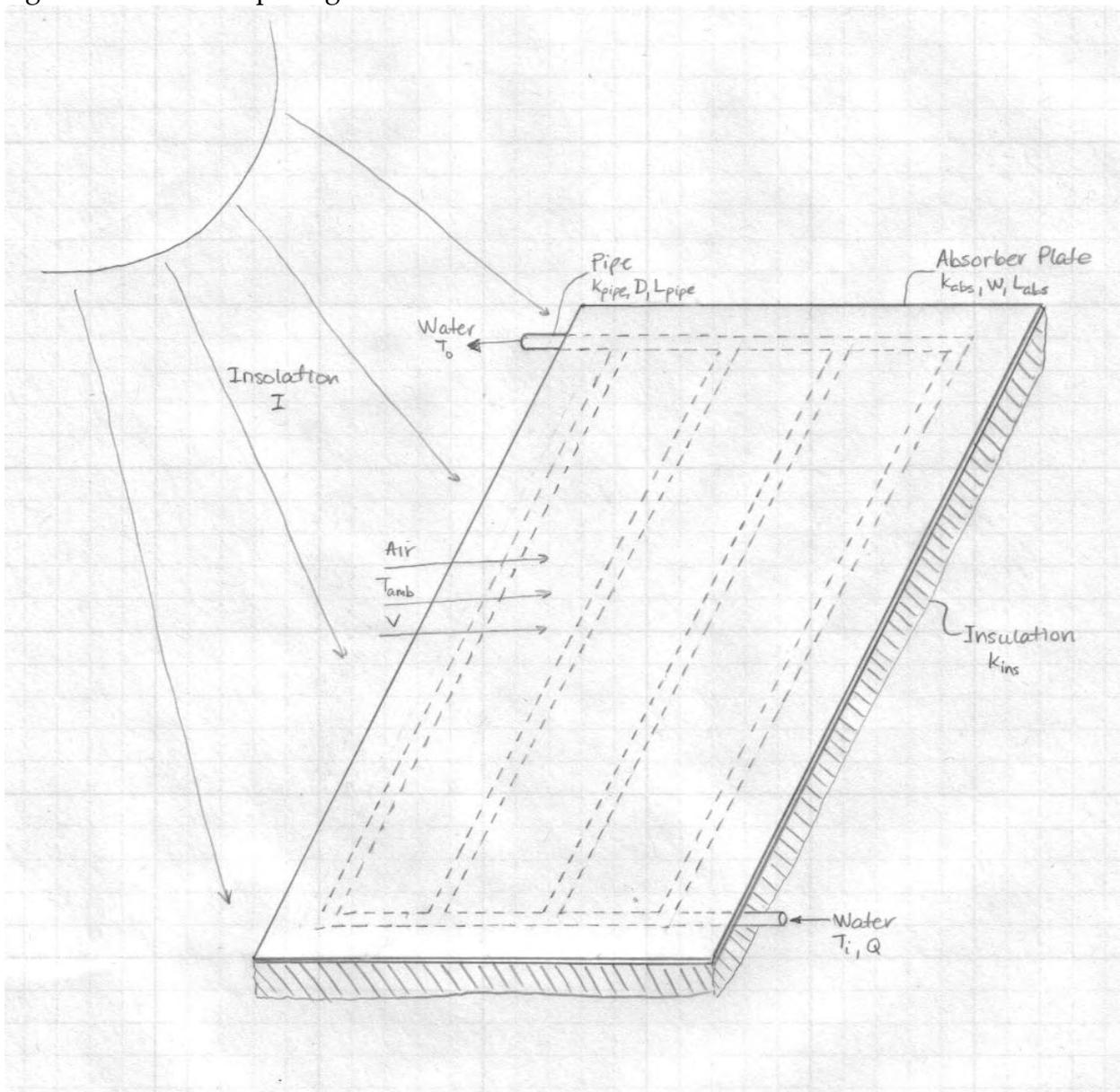
Figure 10: Test 3 Collector Panel and Enclosure Designs
