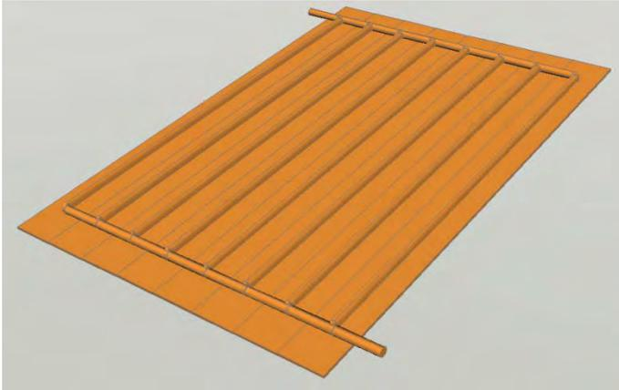
a. parallel pipe array (bottom view)
