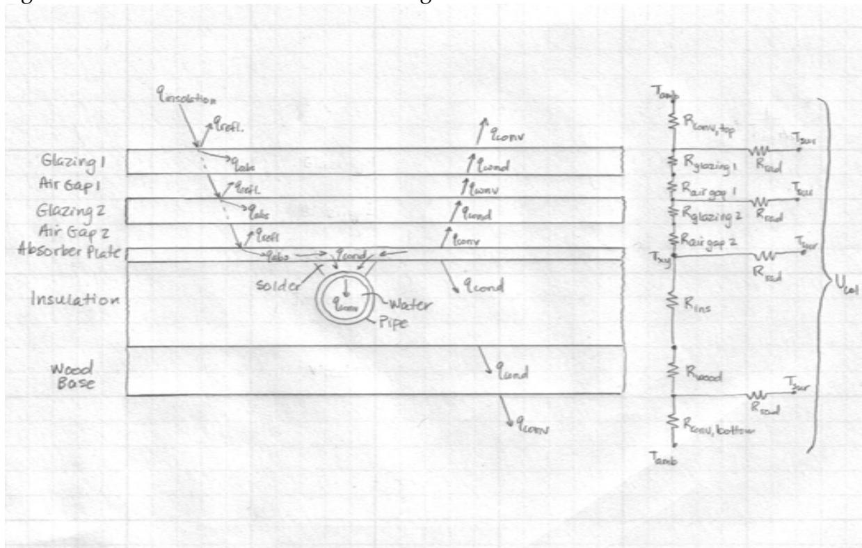
Figure 3: Finite Element Temperature Equation Derivation
