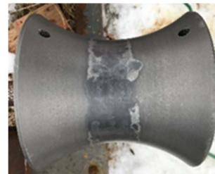
To solve this issue, the capstans were repaired and then anodized, which covered the aluminum in an extremely hard coating. However, additional testing indicated this coating was not effective enough to reduce the wear.
