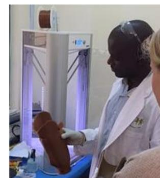
Figure 4 - One of the technicians (Shadrack) holding a printed prosthetic socket next to the 3D printer.
