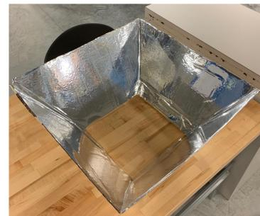
A reflector will sit on top of the glass lid during normal use, but this was removed for the picture. An Excel document has been created to output reflector dimensions based on the efficiency of the pot assembly.
