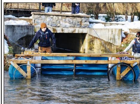
Undershot Water Wheel Mounted on Pontoon—WEDGE 4.2 testing produced 3 watts of mechanical power
